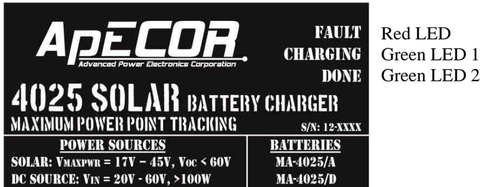
Figure 5: Label on top of charger and LED location
