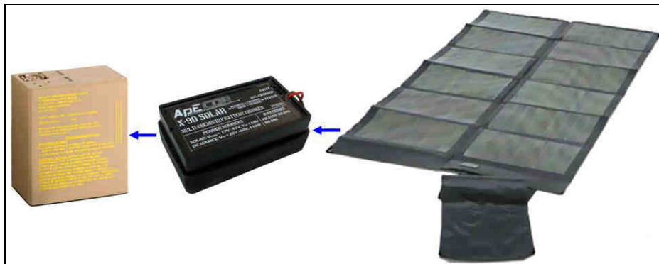
Figure 1: Charger Setup 1 with one Solar Panel as power source
